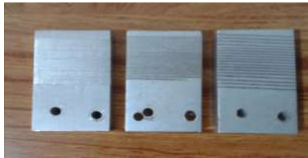
Figure 3. Flat samples for surface roughness measurements
